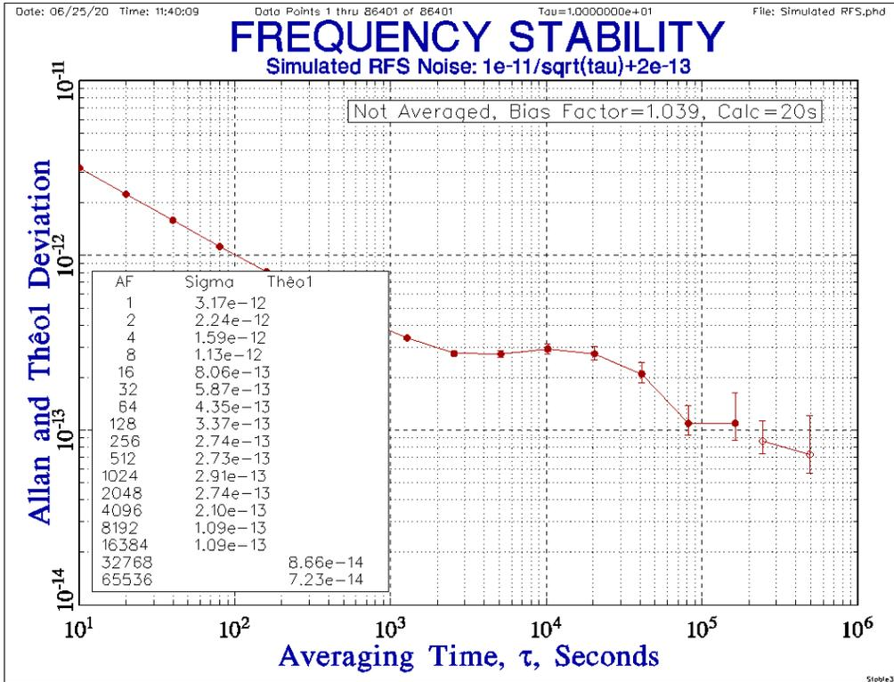
Performing the un-averaged Thèol run in Stable32 at octave tau increments takes only 20 seconds.
