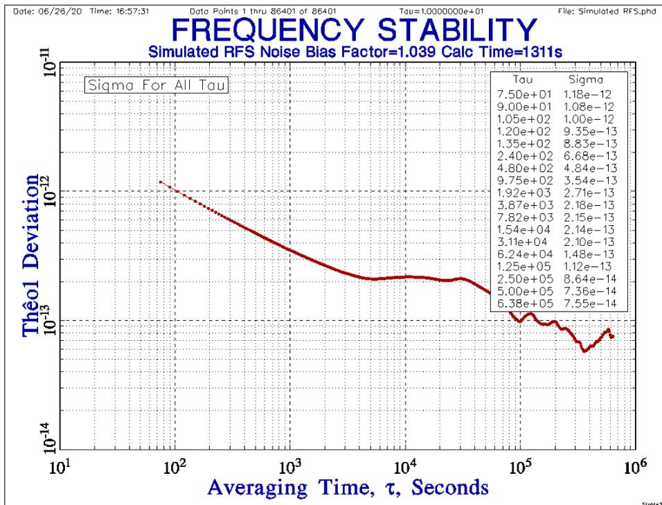
The otherwise same ThêoBR calculation and plot is nearly identical, with a Bias Factor of 1.039 ( $\alpha=0$ , W FM noise) and calculation time (1311s), and, for practical purposes, the same as the R results.
