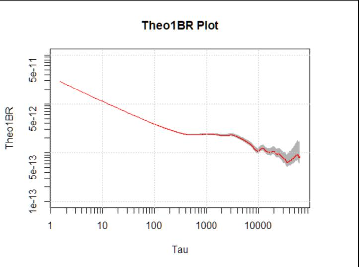
This function was invoked for the 1001-point phase data test suite with the confidence interval set to 95% to emphasize the error bars. The resulting ThêoBR plot is shown below where the grey shading denotes the 2-sigma (95%) confidence interval region. More elaborate plot formats are, of course, possible. The ThêoBR bias factor was 1.085666 (W FM).
