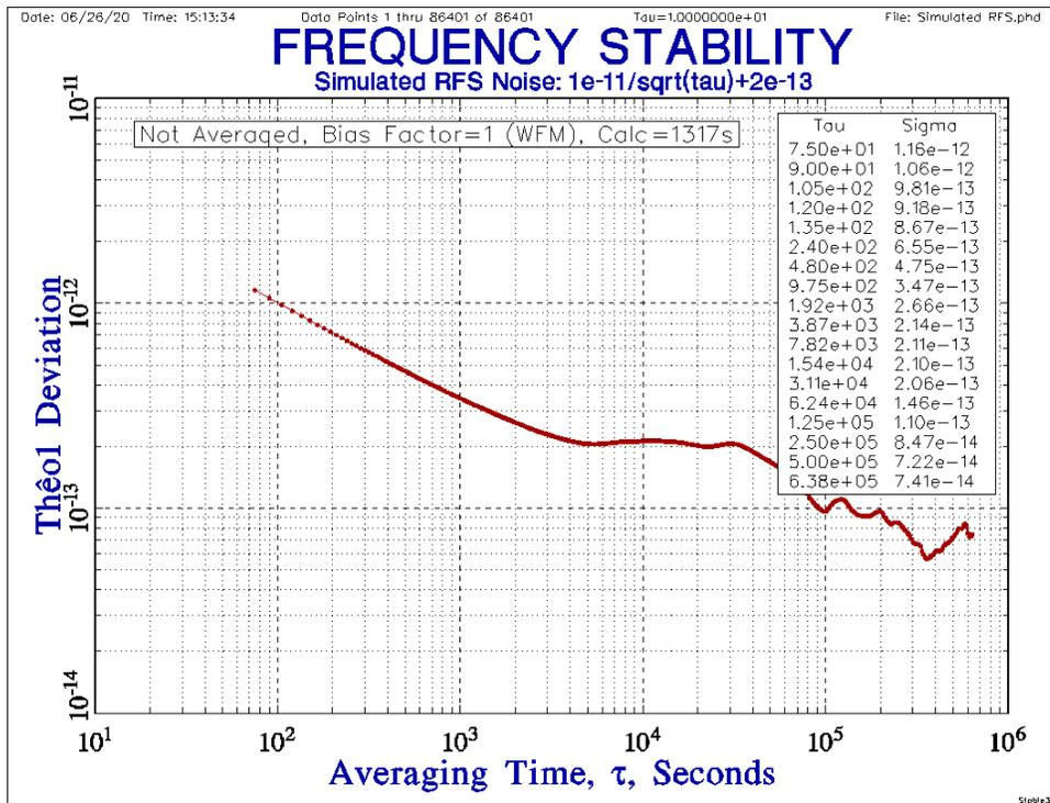
This basic 86,400 point All Tau Thêo1 calculation (no bias removal or error bars) in R using the Lewis fast algorithm takes about 5 seconds, while the same calculation using the naïve method in Stable32 takes 1317 seconds (22 minutes), about x260 times longer. An All Tau Thêo1 calculation takes longer than a ThêoH calculation because most of the points are ADEV values in the latter.
